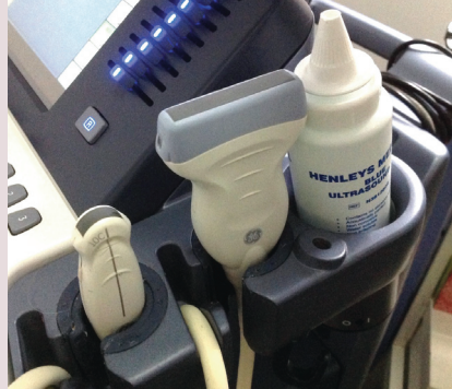
Figure 2 Transducers used for feline abdominal ultrasound by the author. The transducer on the left is a microconvex type, easily recognised by its small, curved footprint. On the right, the linear transducer has a large, flat, rectangular footprint enabling it to provide excellent detail of superficial structures in the near field of the image
